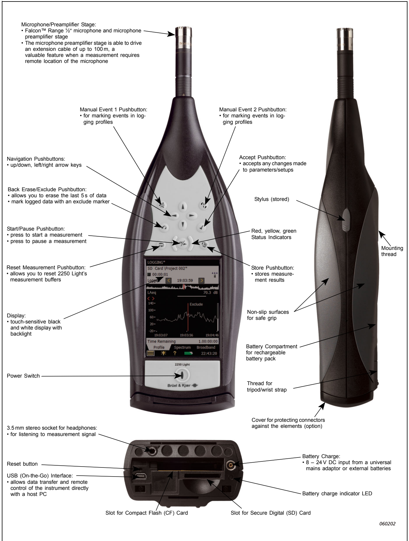
Fig. 1 Key features of 2250 Light
