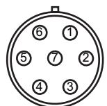
Cable's output plug seen from outside
